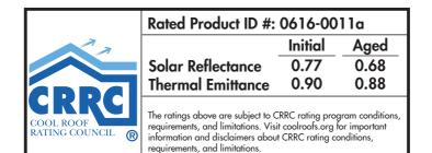
Solar Reflectance Index (SRI) Initial: 96 Weathered: 83
