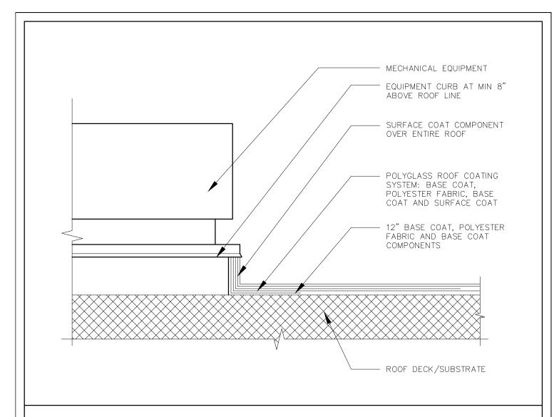
POLYBRITE 70 OR PG 700 ELASTOMERIC ROOF COATINGS. APPLY A MINIMUM OF 2 COATS.
