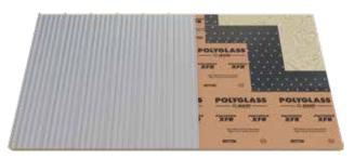
1-Ply + Anchor Sheet UL Class A System: Polystick XFR self-adhered to ASTM D226 (II) 30# Felt anchor sheet onto Plywood under Standing Seam metal
